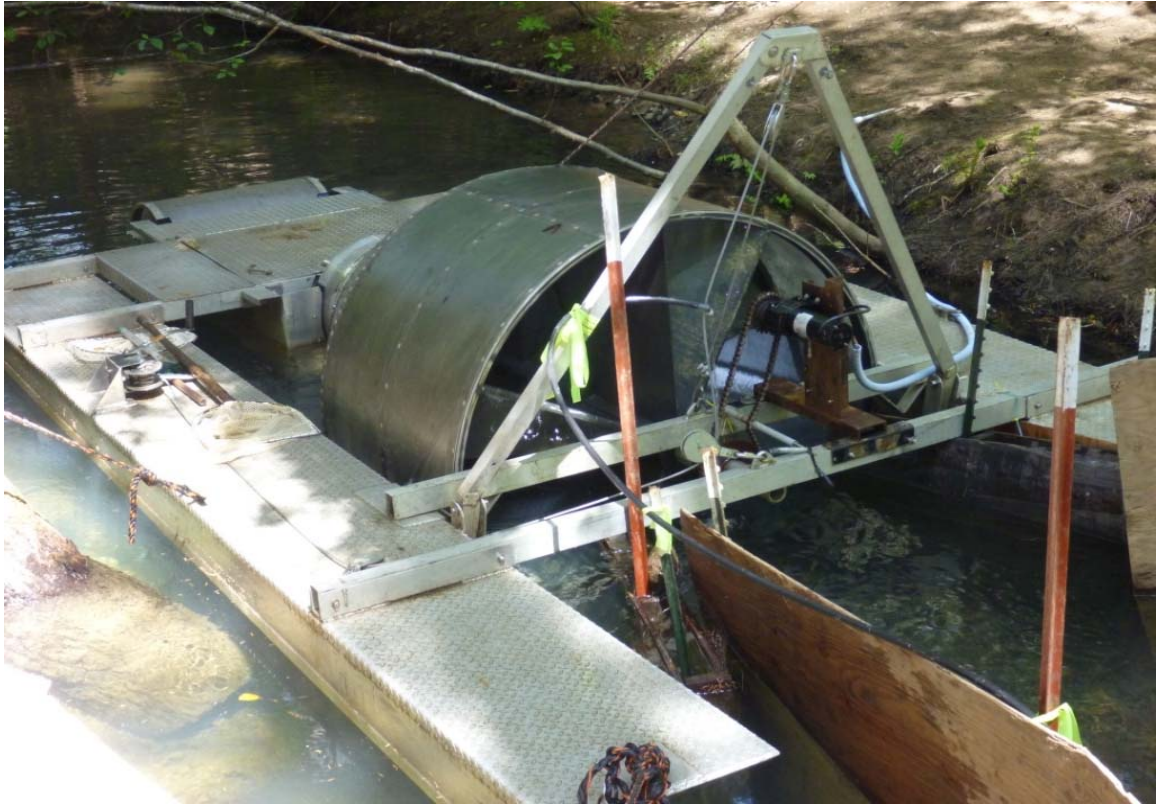
Figure 2. A motorized rotary screw trap in the Little North Fork Navarro River 2011.
